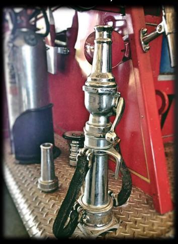
Attack lines were commonly fitted with tip sizes that included 1", 1  $^{1}/_{8}$ ", and 1  $^{1}/_{4}$ "; eventually, these began being manufactured in a stacked tip configuration.
